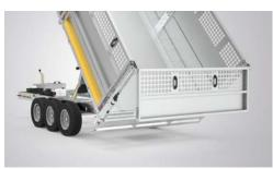
O High panelled side extension kits enable the transport of bulkier loads. Light weight, yet robust panels can be individually removed, along with the quick release retaining posts. This enhanced functionality makes **Tipper2** easily configurable.
