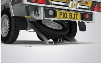
• Spare wheel stored in rear under tray, released from the rear without having to tip the load.
