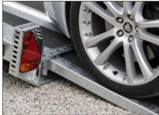
**Easy slide ramps** deploy in only a few seconds, are captive so can't be fully withdrawn. The ramp system facilitates the low loading ability.
