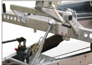
**Powerful Hydraulics** used to lift the tilt-bed version into position for loading. This facility provides a loading angle suitable for low sports cars.
